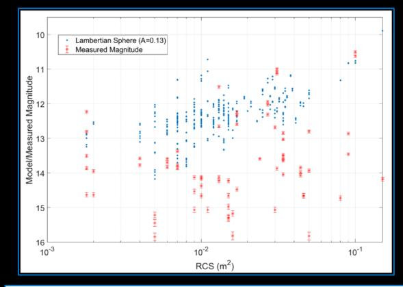
Figure 2 – Fengyun 1C debris measured with JTMA image stacking, showing measured magnitude vs radar cross section.
